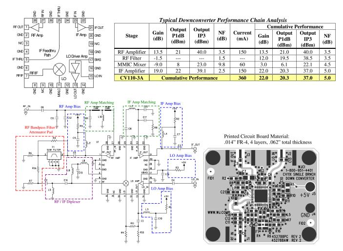
**CV110-3A**: The application circuit can be broken up into four main functions as denoted in the colored dotted areas above: RF/IF diplexing (purple), amplifier matching (green), filtering (red), and dc biasing (blue). There are various placeholders for chip components in the circuit schematic so that a common PCB can be used for all WJ single-branch converters. Additional placeholders for other optional functions such as filtering are also included.
